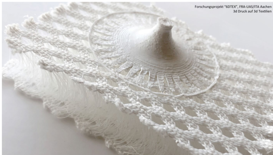
Fig. 13 6dTEX, 3D printing on 3D textiles, Frankfurt UAS together with ITA Aachen. © Frankfurt UAS
