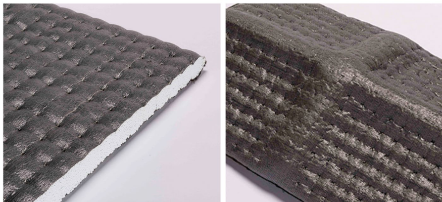
Fig. 8 Composite building component from expanded rPET particle foam in combination with lost formwork from rPET fiber—woven spacer fabric; left—planar element; right—self-foldable, formative element. © Frankfurt UAS
