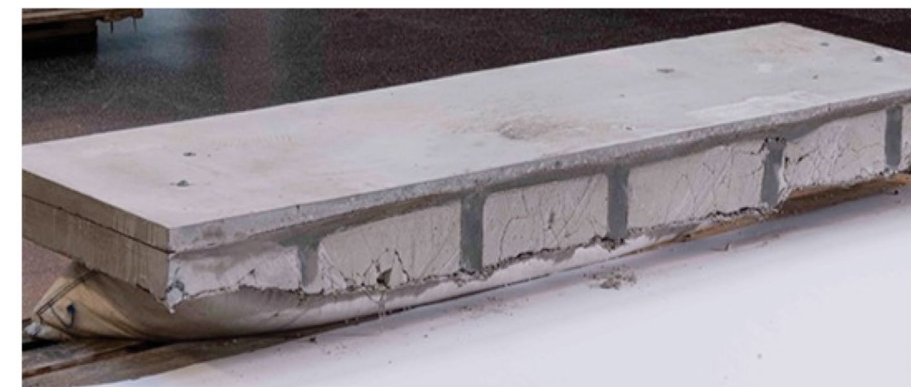
Fig. 6 First demonstrator: Formative composite building component made of ultra-high performance concrete (UHPC), with lost insulation formwork made of basalt fiber spacer fabric, formed by a cement foam filling. © Frankfurt UAS
