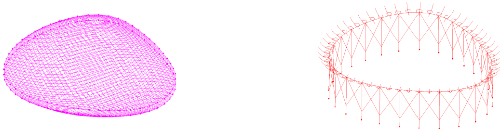
Figure 4: Divided overall system. Left membrane, right steel ring with supports and cables.
